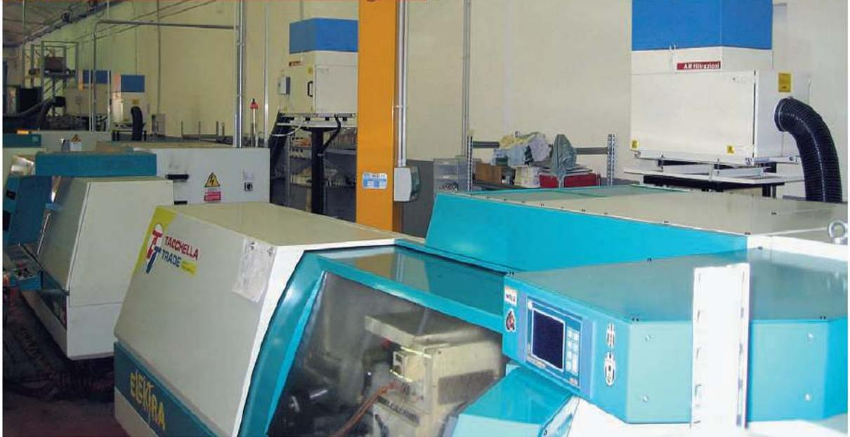
**The air cleaners of the series ARNO VF are suitable for the removal and purification of oil mist and dust produced during wet and dry machining processes. Here is an example of an installation on grinding machines.**
