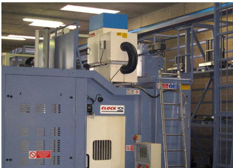
**Example of an application of an air cleaner ARNO VPF on a machining centre at BETTINELLI S.p.A.**
